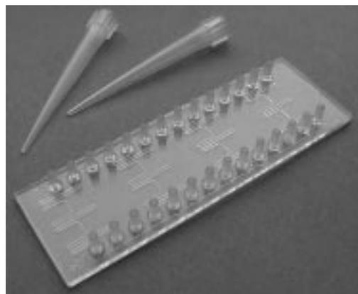
**Fig. 14:** PCR chip with freely programmable number of cycles.
