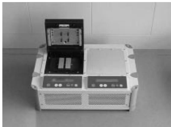
**Fig. 4:** Chip thermocycler unit which can be equipped with two PCR chips simultaneously.
