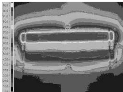
**Fig. 7b:** Thermal distribution after a 250  $\mu\text{m}$  cover foil.
