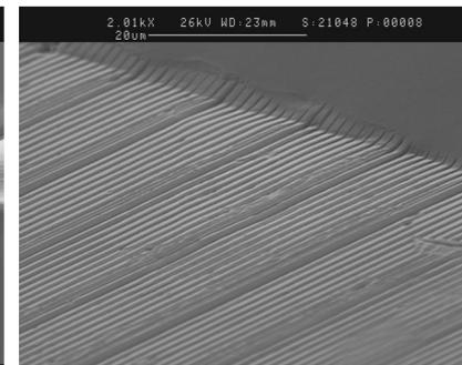
**Fig. 5c:** Close-up of the area channel-wall and nano-structure. The structures are not as well replicated as in the case of COC.
