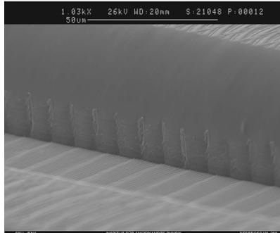
**Fig. 4b:** Close-up of the area channel-wall and nano-structure.
