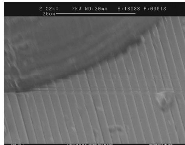
**Fig. 7b:** Detail of the nanostructure. The resolution of the SEM could not be as high as in the case of COC as thermal damage in the PMMA could be observed due to the electron beam.
