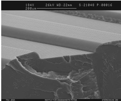
**Fig. 4a:** Overview of injection molded COC. Note the rounding of the micro-structured channel wall due to incomplete mold filling.
