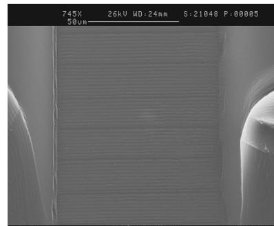
**Fig. 5b:** Close-up of a single channel with nanostructures.
