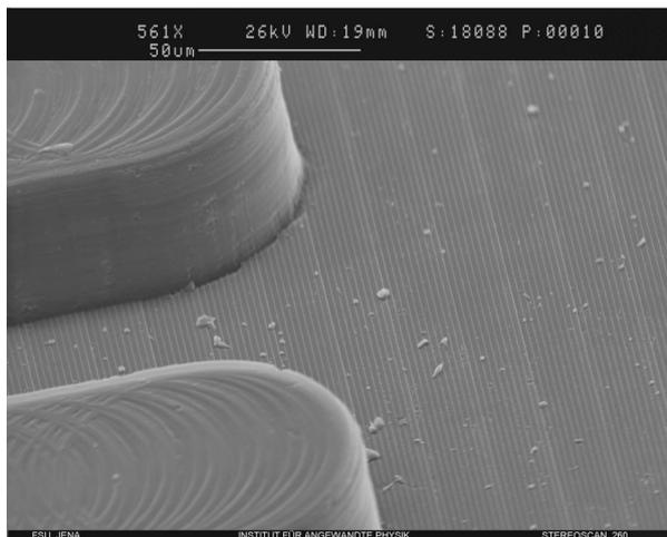
**Fig. 7a:** Hot embossed structure in PMMA. Note the high replication accuracy both of the micro- as well as the nanostructure.
