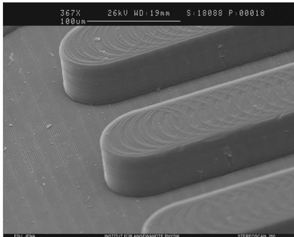
**Fig. 6a:** Hot embossed structure in COC. Note the high replication accuracy both of the micro- as well as the nanostructure.
