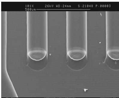
**Fig. 5a:** Overview of injection molded PP. Note the rounding of the micro-structured channel wall due to incomplete mold filling and some deformation at the ends due to demolding.
