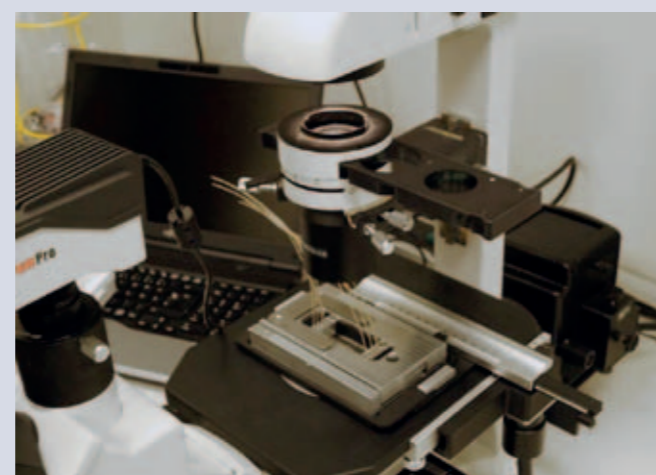
Lab-on-a-Chip Cell Culture Incubator – LOC CCI 1 placed on a microscopy stage
