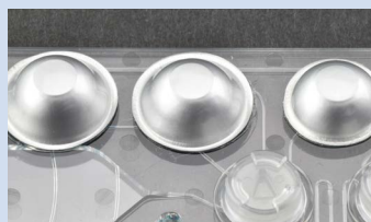
Liquid reagents stored in blisters
