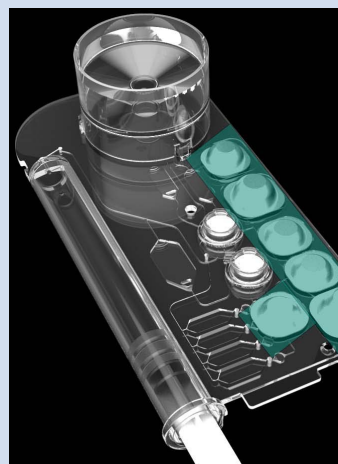
Metering of the sample and incubation with assay reagents on chip
